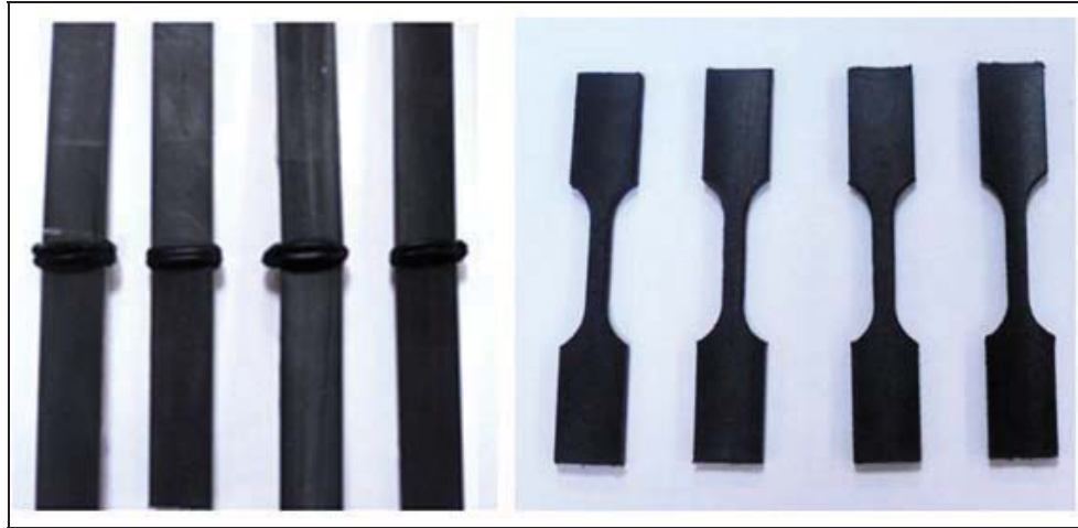
Figure 3: (a) Fusion welded HDPE strips, (b) Machined fusion weld tensile samples
