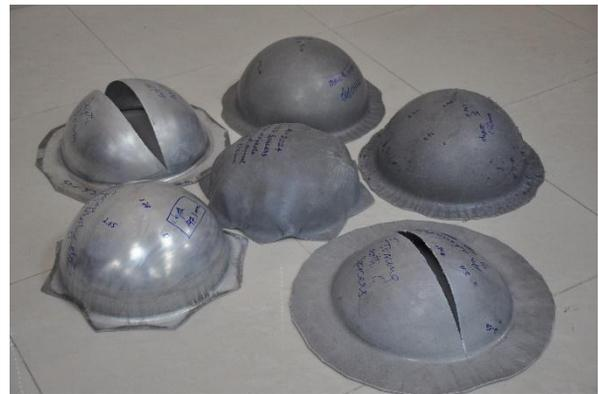
Fig. 1. Images of formed (fractured/non-fractured) hemispheres
