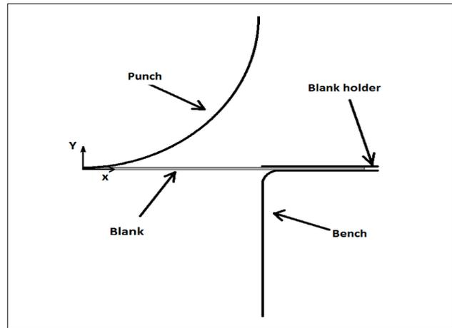
Fig. 4. Axisymmetric representation of the forming process
