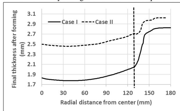
Fig. 6. Thickness reduction of the blank due to forming with different friction conditions
