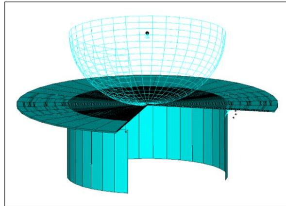
Fig. 5. Finite Element Model for forming simulation
