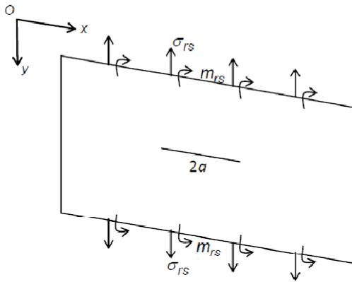
Figure 4 - The bending and tensile stresses for a part-through crack of length 2a, after Rice and Levy [13]
