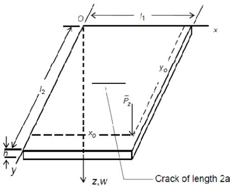
Figure 5 - Isotropic plate having a small crack at the centre under the application of point load at some arbitrary position [6]
