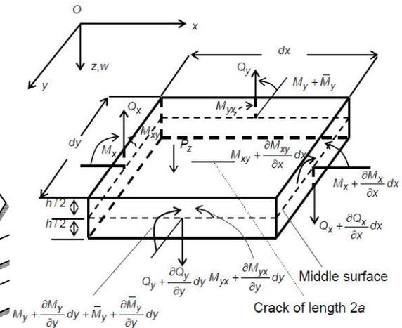
Figure 1 - Isotropic plate loaded by uniform pressure and a small crack at the centre
