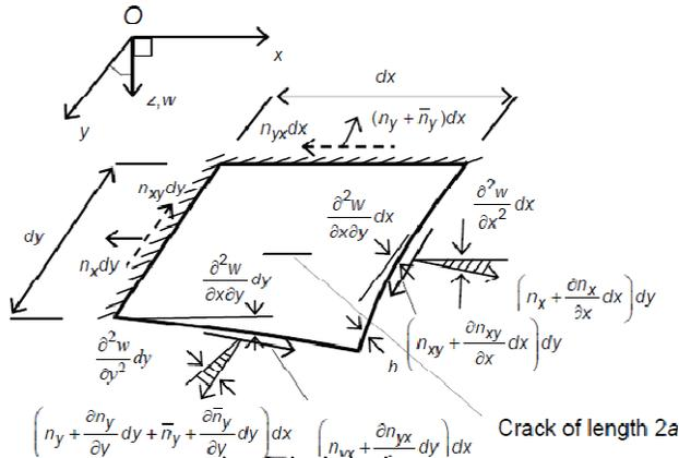
Figure 3 - Two sided constraints and plate deformation having a part-through crack at the centre
