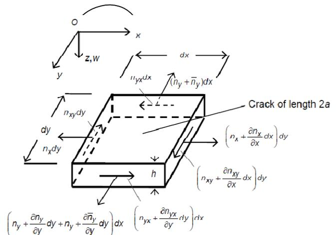
Figure 2 - In-plane forces and a crack of length  $2a$  at the centre of the plate element
