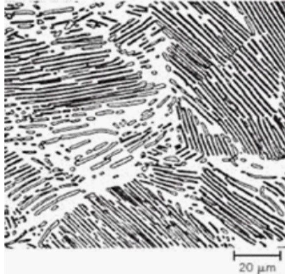
Figure 1.5: Pearlite in steel consists of two phases, ferrite and carbide.
